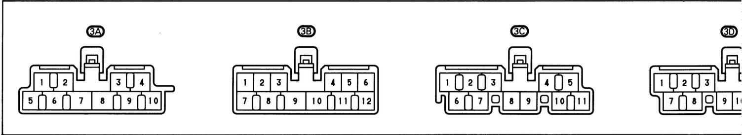
**Connector Joining Wire Harness and Wire Harness
