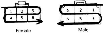
The numbering system for the overall wiring diagram is the same as above.
