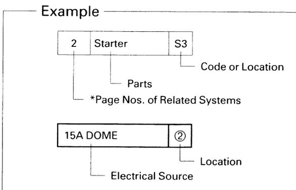
\* These are the page numbers of the first page on which the related system is shown. The part indicated is located somewhere in the system, not necessarily on the page indicated here.
