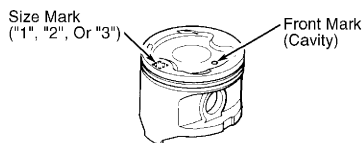
Fig. 54: Identifying Piston Size Marks Courtesy of Toyota Motor Sales, U.S.A., Inc.
