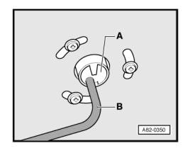
Remove any residue from auxiliary/additional heater combustion chamber (this is particularly important for vehicles with diesel engines and when running engine and thus auxiliary/additional heater on rape-oil or vegetable-oil methylester fuel)
