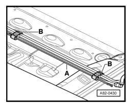
In area behind front right wheel housing liner, fuel pipe to auxiliary/additional heater -A- is routed as illustrated for vehicles with petrol engine (routing may differ from that shown in the case of vehicles with diesel engine).
