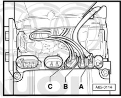
Measure the resistance at connector -C- between contacts "11". Copyin and "2". permitted unless authorised by with respect to the correctne
